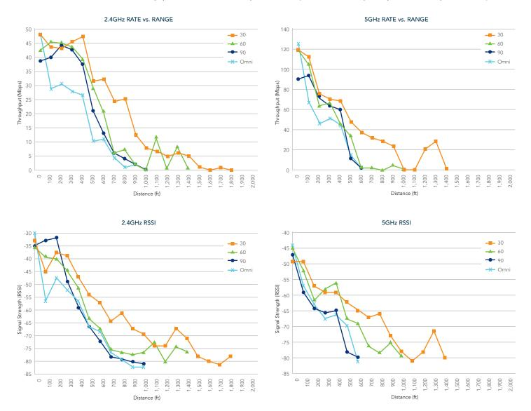
Note: the Omnidirectional antenna used in these tests is the ANT-OMNI-2x2-02 not the Rubber Duck Antenna.
